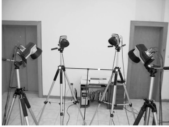
图 2 4 台摄像机组成的标定及测量实验系统实物图 Fig. 2 Experimental calibration and measurement system composed of four CMOS cameras
